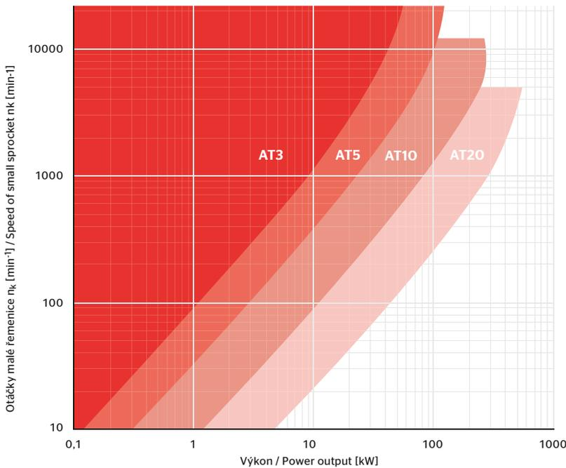
Various factors have to be considered when choosing the correct ContiTech timing belt. The timing belt selection graphs below will help identify the correct belt for your application. A selection of the commonest belt types is shown.
